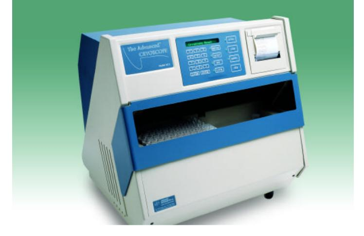
Such an instrument can check the freezing points of samples of size 2ml to help determine whether milk has added water in it. Ordinarily milk already is 88% water, we are talking about added water contents here. Added water raises the freezing point milk.
